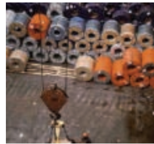
Left: Tanktop after coil loading.
