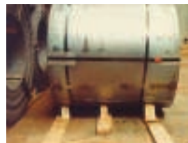
Figure 1 – Dunnages create patch loads on the tank top
