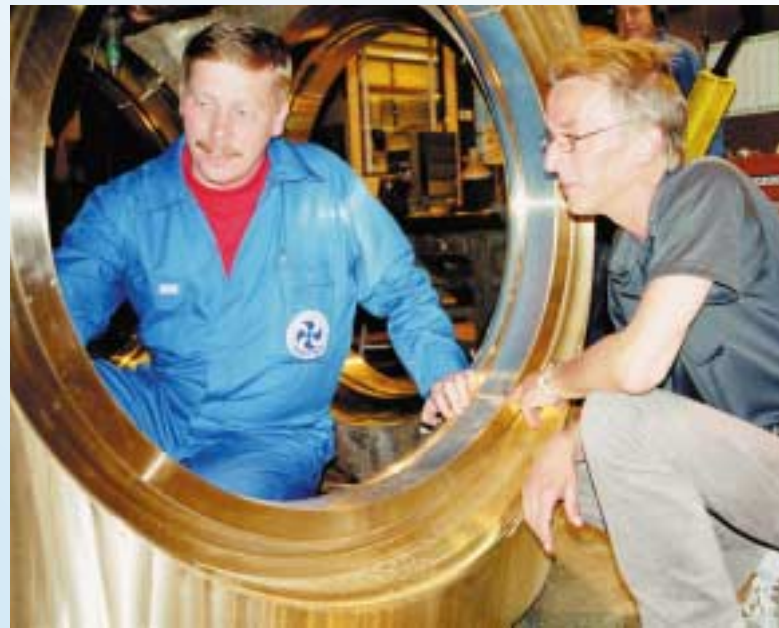
Lars Olav Lindalen, DNV surveyor, and Göran Karlsson, head of classification at Rolls-Royce AB, inspect the packing surface of a propeller boss due for delivery to Italy's Fincantieri shipyard. When finished, the propeller will weigh 76 tonnes and have a diameter of 5.7 metres.
